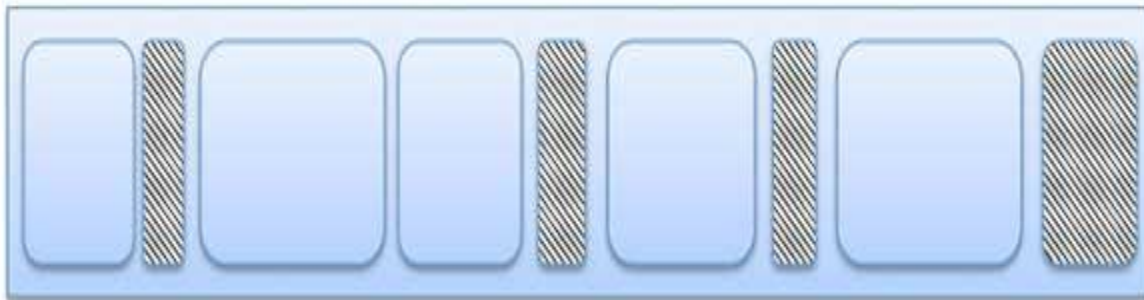
Fragmented memory before compaction
